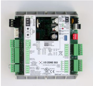
Figure 1: Direct Digital Controller
